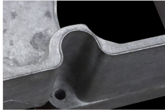
When subjected to the same test, a Delphi K-Alloy casting shown above exhibits virtually no signs of corrosion.
