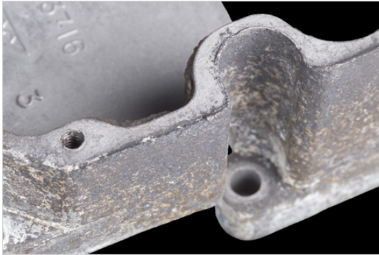
The image above shows the corrosion level of a conventional A360 aluminum casting when subjected to a 30-day salt spray test.
