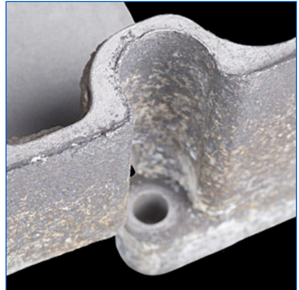
Corrosion level of a conventional A360 aluminum casting when subjected to a 30-day salt spray test.
